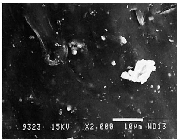
Figure 6 SEM micrograph of calcium carbonate in PE (fracture surface).
