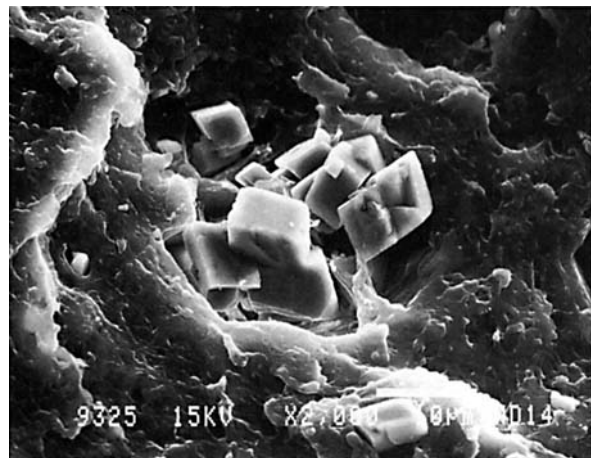
Figure 5 SEM micrograph of calcium carbonate in PS (fracture surface).
